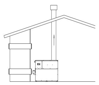
FIG. 8 Outside Combustion Air Through Ducts
